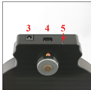
3- Power input; 4- USB socket; 5- Motor tension adjustment
