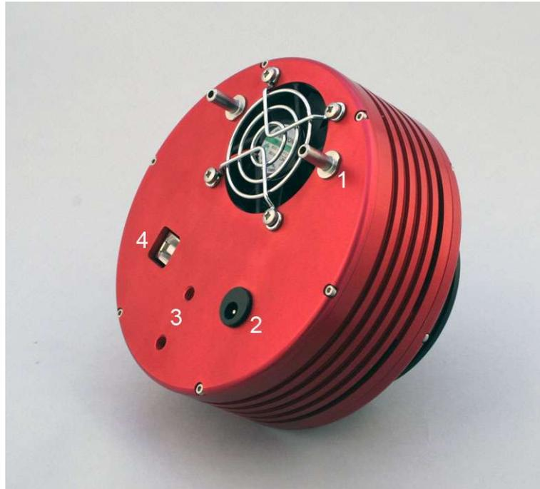
1. Water cooling pipes
