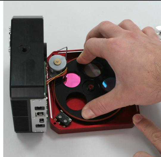
Install disk. Make sure the disk clears the mechanical index on the lower left. If needed, use a pen tip to lower the blade.
