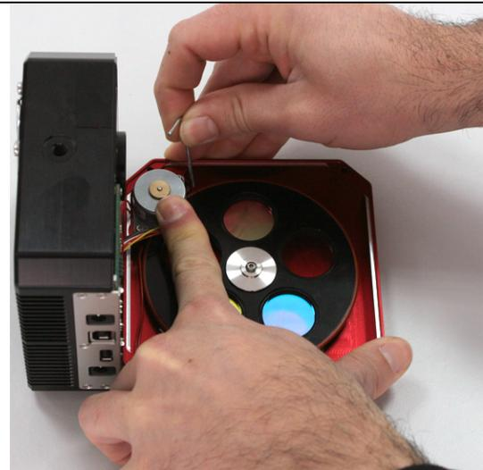
Place the top bearing in place and the washer as well. Tighten back the screw, and make sure the wheel rotates well, rotating to the right.
