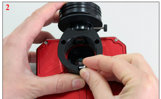
2- Align the module with the 3 holes and attach it to the Atik One camera, using the 3 supplied screws.
