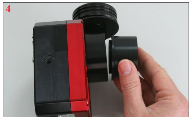
4- Screw back in the 2" adapter onto the module.
