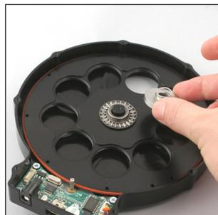
To remove the disk, take the spring, metal bushing and bearing off.
