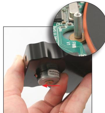
Push the motor in the direction of the USB socket. Note that the shaft will detach from the rubber.
