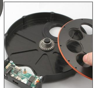
Take the disk off while pushing the motor. To install the new disk, repeat the process in reverse. *Make sure the cover is put back in place in an up-down motion, to avoid bending the central spring.*
