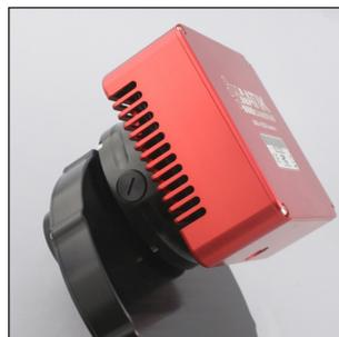
Insert the camera with the adapter into the EFW2 and screw in the two retaining grub screws.
