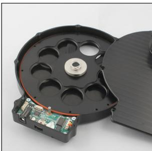
Unscrew the screws and take the cover off. Install filters in the numbered slots.
