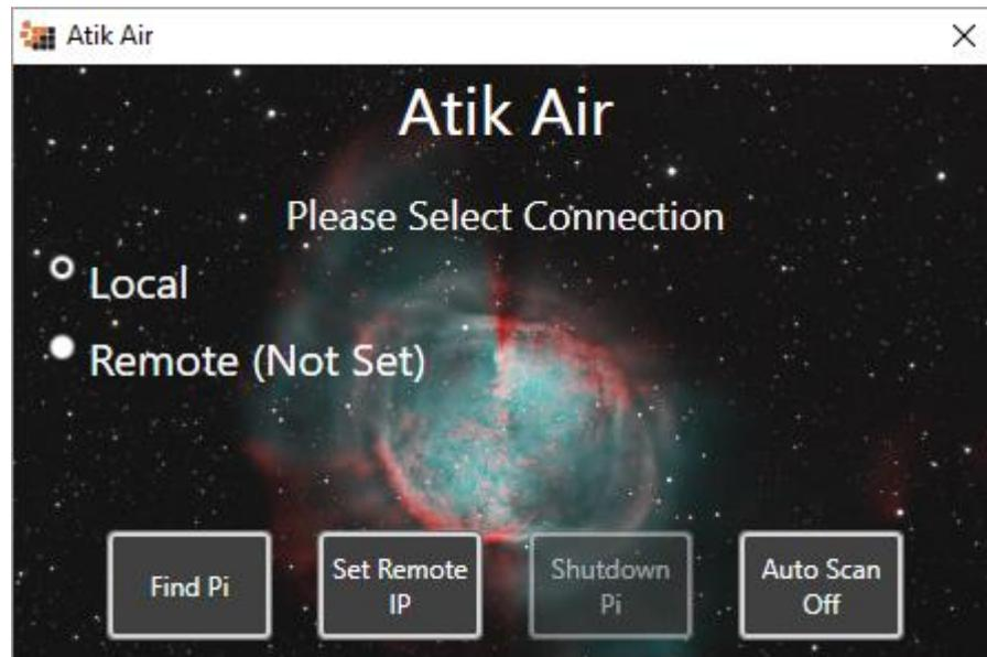
*You will see two options 'Local' and 'Remote'. Local will look for cameras connected to your PC. Remote will look for cameras connected to the Raspberry Pi. The first time you see this screen, Remote will say 'Not Set'. Before you can use the cameras connected to the Raspberry Pi, you will need to set it up.*
