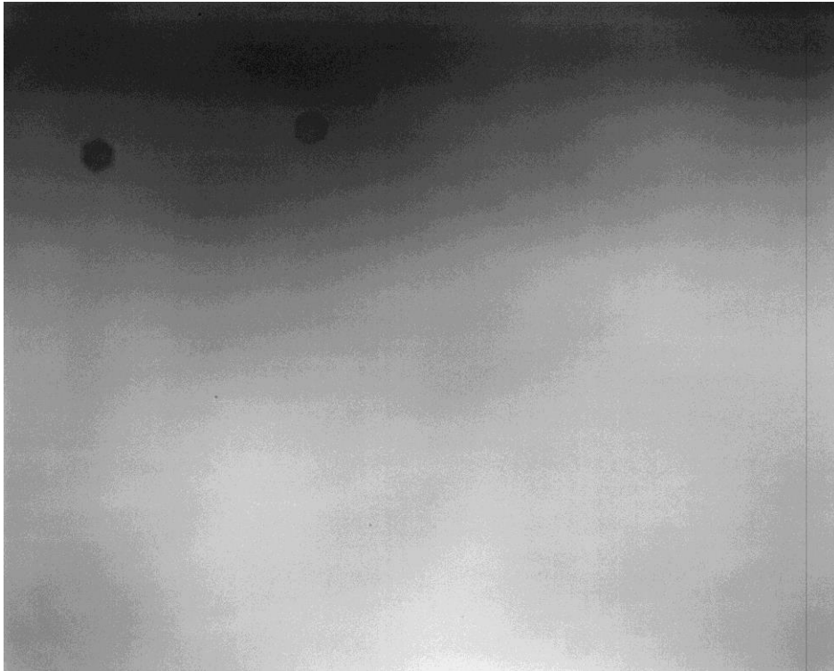
Flat field from 16200 showing column defect before correction
