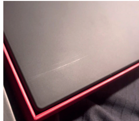
Varying the illumination angle can make it easier to spot subtle defects where contrast is poor
