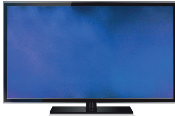
An example of screen Mura – in this case showing noticeable luminosity variation in different areas of the panel
